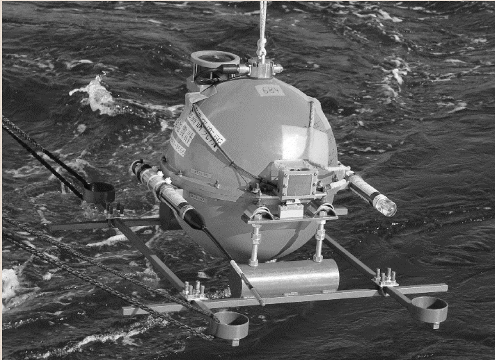
Figure 2. Photograph of a long-term ocean bottom seismometer just before deployment Orange sphere is made of titanium alloy and contains equipment for seismic observation.
