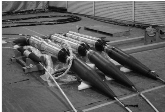
Figure 8. Photograph of observation units of the OBCST system, which was deployed off Sanriku, Japan in 2015
