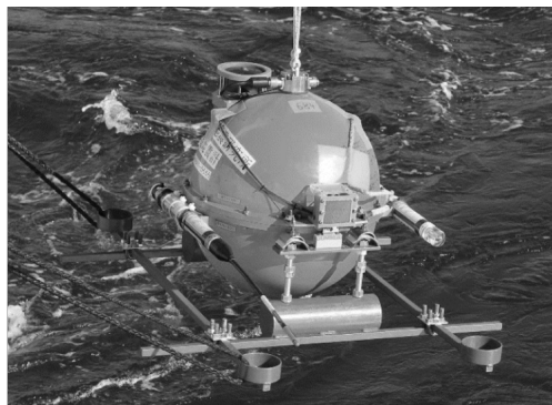
Figure 2. Photograph of a long-term ocean bottom seismometer just before deployment
